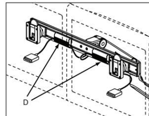
*Note: For dual-monitor applications, first route monitor cables through cable management clips (D), then refer to Step a.*
