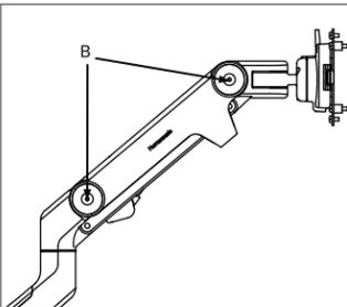
Use Hex Key B to turn the screws on each friction disc clockwise to increase friction. Turn each screw counterclockwise to decrease friction. Be sure to apply the same amount of rotation to each screw.
