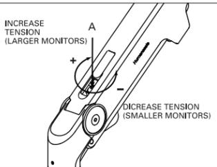
Use Hex Key C to adjust the Tension Screw (A) located in the Upper Arm of the M8. Turn the Tension Screw clockwise to increase tension for larger, heavier monitors. Turn the Tension Screw counterclockwise to decrease tension for smaller, lighter monitors.
