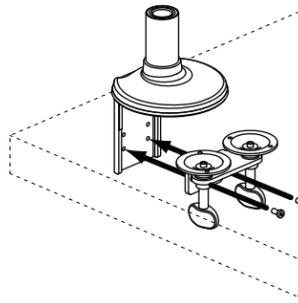
*Note: There are two sets of Bracket Screw holes to accommodate different surface thicknesses. Use the set of holes that allow the Clamp Screws to tighten fully. Use the top holes for surfaces up to 1.8" (48mm) thick and lower holes for surfaces up to 2.7" (68mm) thick.*
