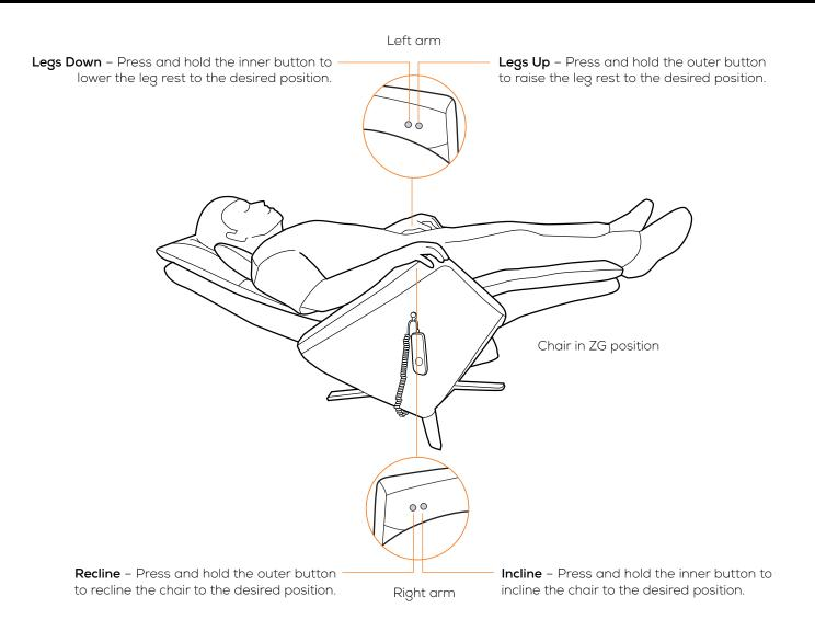
Press the two right-hand in-arm control buttons simultaneously for at least five seconds to lock all in-arm buttons. Repeat to unlock.
